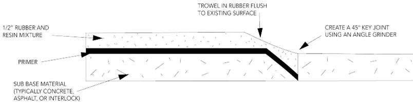
*Figure 5. Installing flush with adjacent surfaces.*
