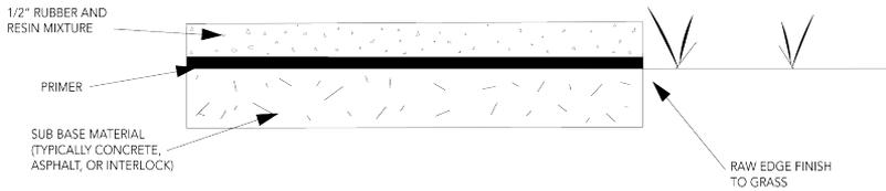
*Figure 2. Installation with raw edge.*
