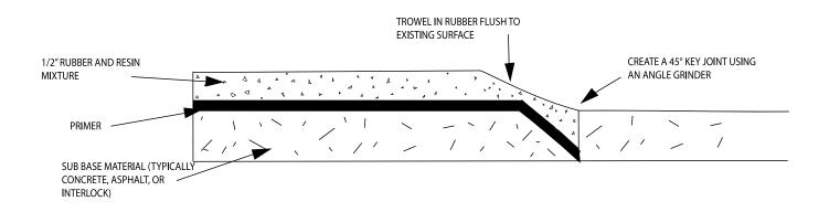
Figure 5. Installing flush with adjacent surfaces.
