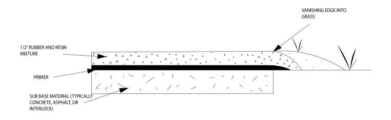
Figure 4. Installation with vanishing edge.
