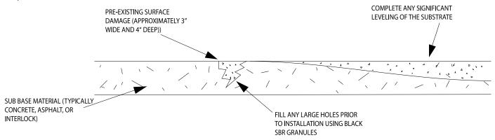
Figure 7. Completing repairs using fill prior to installation.
