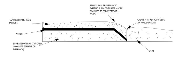
Figure 6. Finishing to curb.
