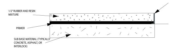
Figure 2. Installation with raw edge.
